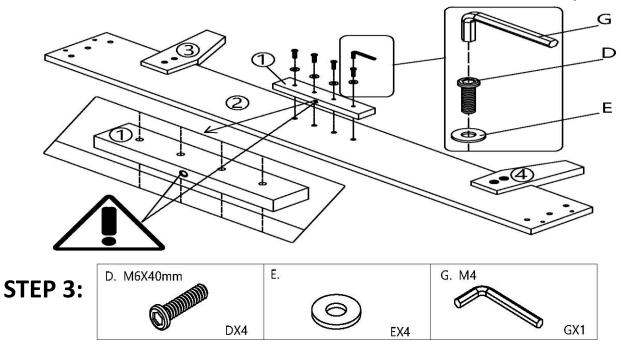
Attach headboard legs (13) to headboard (12) with bolt (D) and washer (E)using allen key (G)
